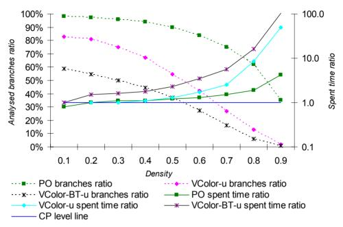
Figure 19. Concluding view on unweighted maximum clique finding algorithms' performance on random graphs
