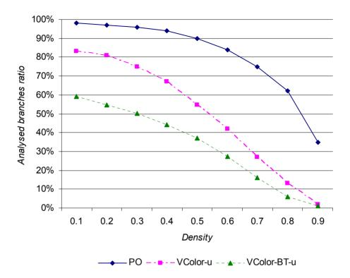
Figure 18. Unweighted case / Benchmark results at random graphs – Analysed branches ratios
