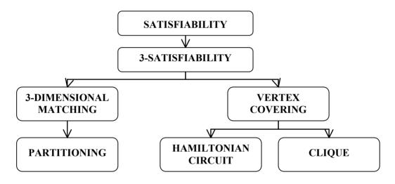
Figure 1. The sequence of transformation of the six basic problems' NP-completeness proving
